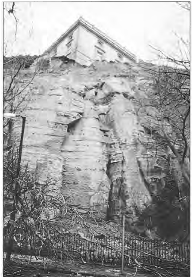
The site of the failure seen from the foot of the cliff on 27th December, before the loose debris was removed, and with the fallen tree and lamp post still leaning across Peveril Drive (photos by Tony Waltham).
